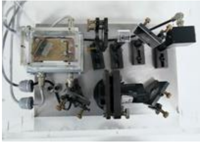
The experimental setup for locking of portable ECDL to the D_2 energy transition of Rb atoms ( \lambda=780 nm)
