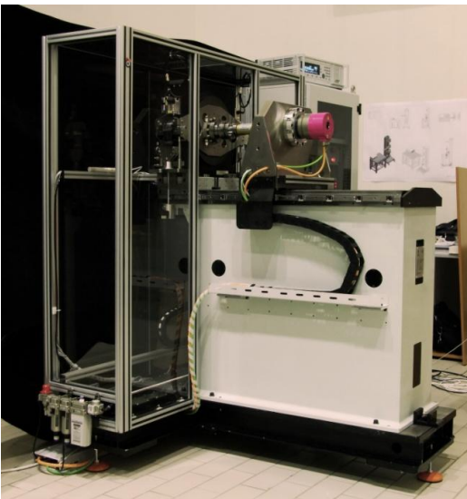
50 N.m Primary Torque Calibration Machine with Lever and Deadweight
