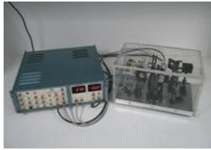
The experimental setup for locking of portable ECDL to the D_2 energy transition of Rb atoms ( \lambda=780 nm)
