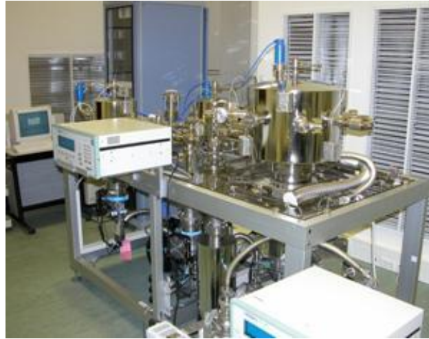
TÜBİTAK UME Primary Vacuum Standard (MSSE1)
