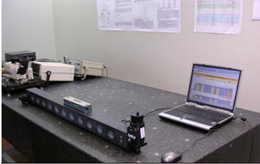
TÜBİTAK UME - 1 Meter Small Angle Generator
