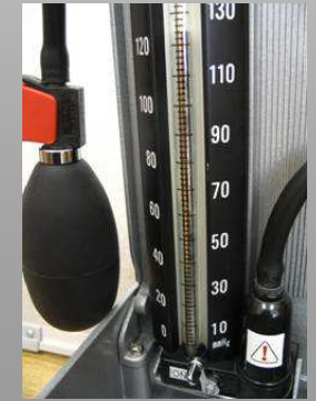
Figure: Measurement setup to determine the limits of error of the cuff pressure indication (home use device)
