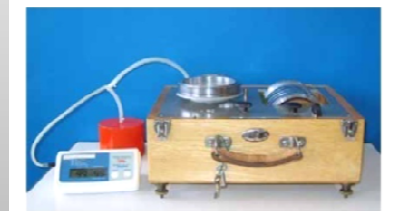
Figure: Measurement setup to determine the limits of error of the cuff pressure indication (home use device)
