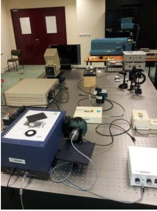
Color measurement setup of reflective, transmittive and emissive surfaces.
