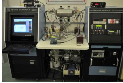
Secondary Level Vacuum Gauge Calibration System (VGMS)
