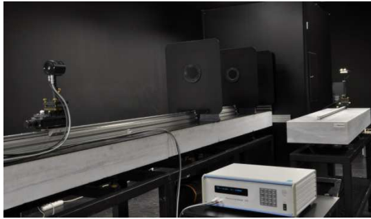
Luminous intensity and illuminance measurement configuration
