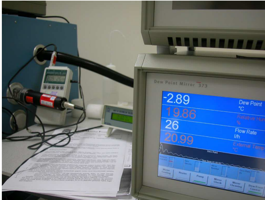
Humidity Calibration Set-up
