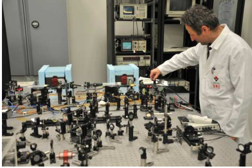
Yb Fiber Based Femtosecond Frequency Comb and Supercontinuum Spectrum Generation in Photonic Crystal Fiber
