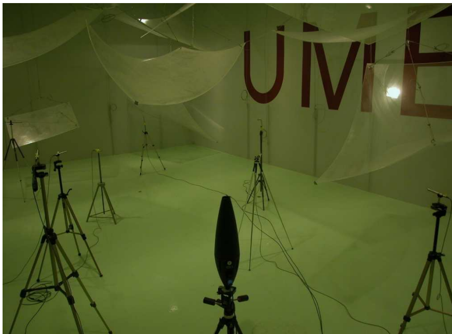
Measurement of the Sound Absorption Coefficient of Material in Reverberation Room
