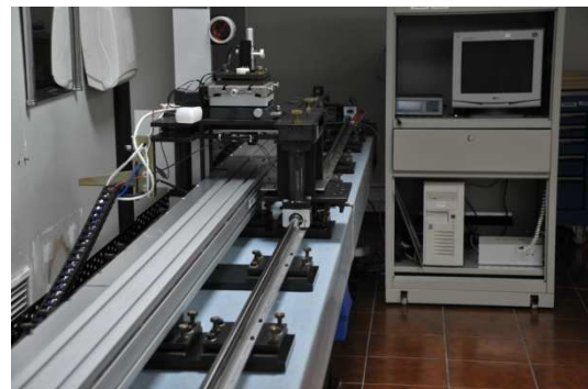
5 m Line Scale and Steel Ruler Measurement System
