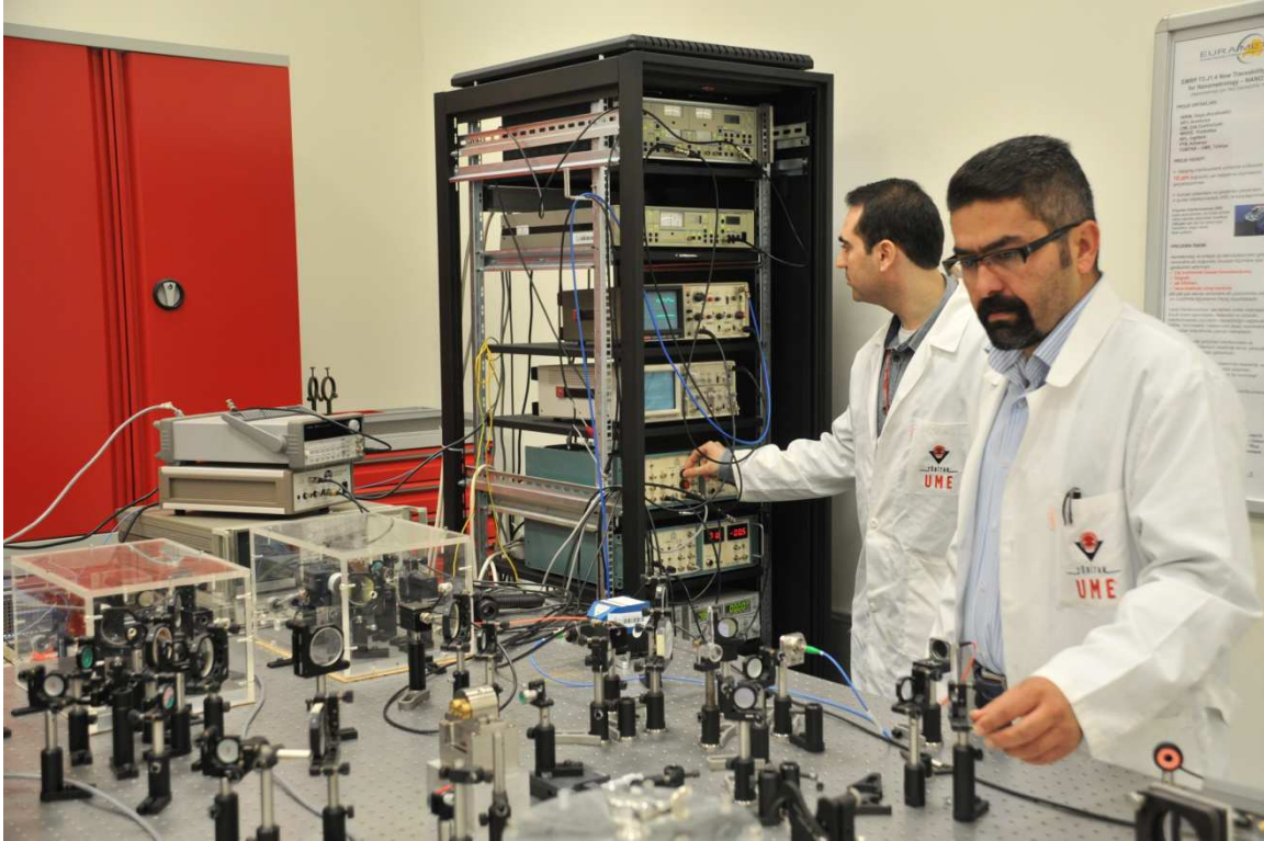
Experimental Set-up for Sub-nanometer Displacement Measurements
