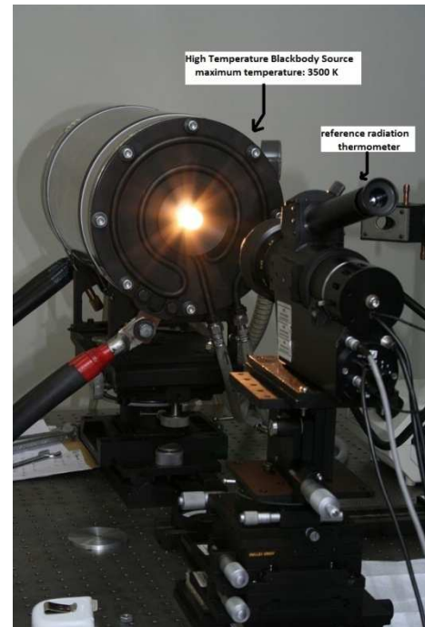
Radiation Thermometer TSP-2 in Front of the Blackbody Source
