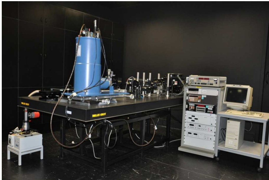
Cryogenic radiometer based-absolute spectral CW optical power measurement system
