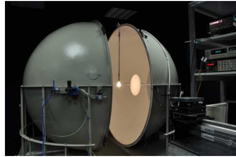
Total luminous flux measurement setup
