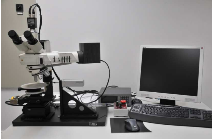
Brinell-Vickers Indentation Measurement System
