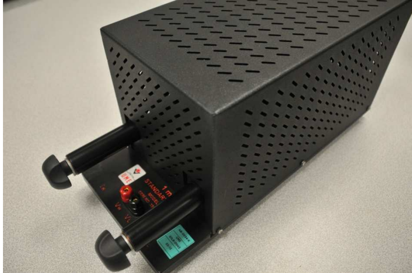
TÜBİTAK UME Made 400\ \mu\Omega Current Shunt
