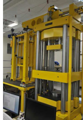
110 kN and 1,1 MN Capacities Force Standard Machines
