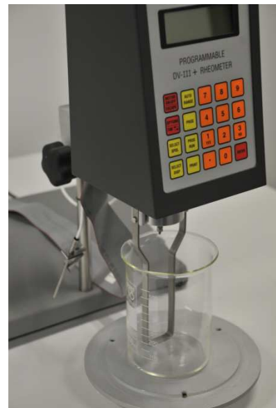
Rotational Viscometer Measurement Setup
