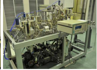
Primary Vacuum Standard "Multi-Stage Static Expansion System" (MSSE1)
